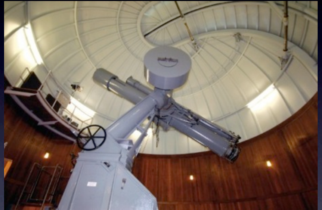
Thompson 26" refracting telescope built in 1896. Focal length: 5.44m 12,169 plates
